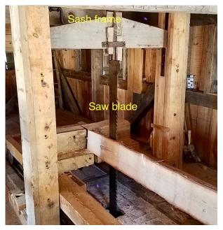
A pusher ratchet turns the rag wheel 6 degrees each time the saw moves up, advancing the log ¼ inch towards the saw blade. A keeper ratchet then locks the rag wheel and carriage while the blade moves down sawing. The pusher ratchet is driven by a wooden linkage connected to the saw frame. You can see the linkage rocking back and forth and hear the steel ratchets clicking during sawing.
