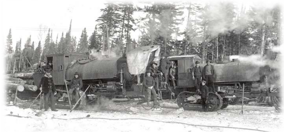
Eastern Manufacturing Lombard log haulers, T9-R14, Circa 1908-1913, O.A. Harkness, Terence F. Harper Collection
