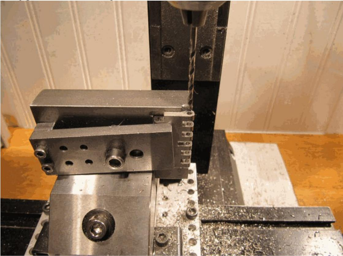
cut roller bearing grooves on inside
