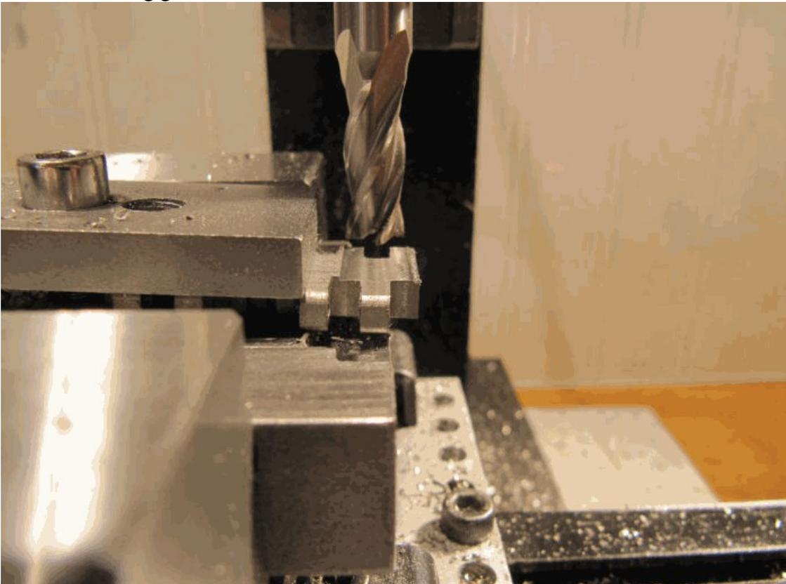
and angle jig to hold for shaping the outside with a ball end mill
