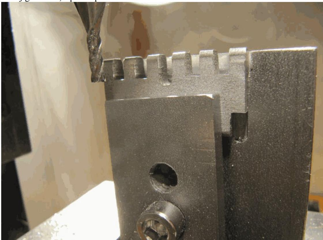
with jig on its side, drill the pivot holes
