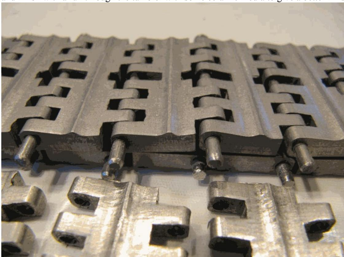
Similar jigs were made for making the chains, riveting, and drilling the pivot pins for the cotters.
