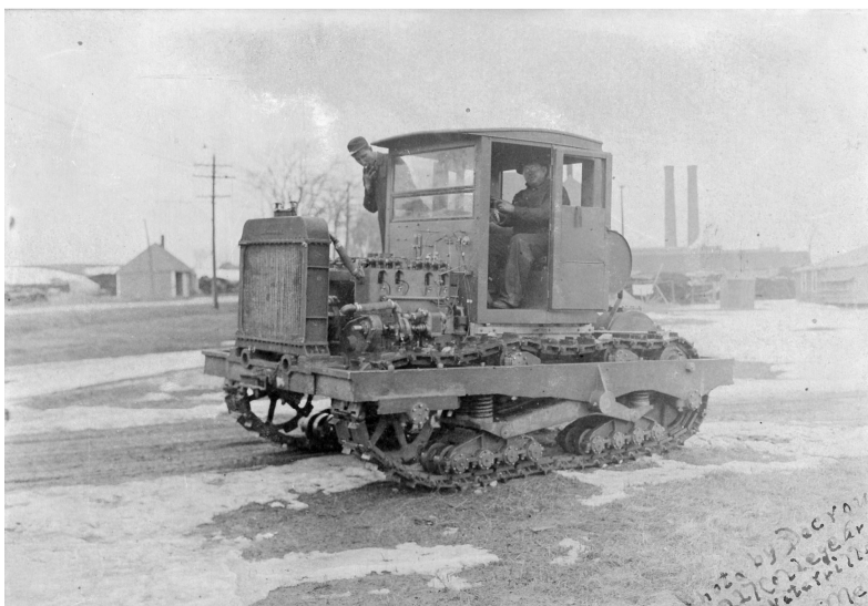
The A-O-L (Old Twin) at the Lombard factory. Note the twin Stearns engines Terence F. Harper Collection
