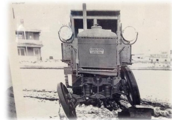
Lombard Model "T" illustrating the flexibility of the front axle. Circa 1927-1928 Terence F. Harper Collection
