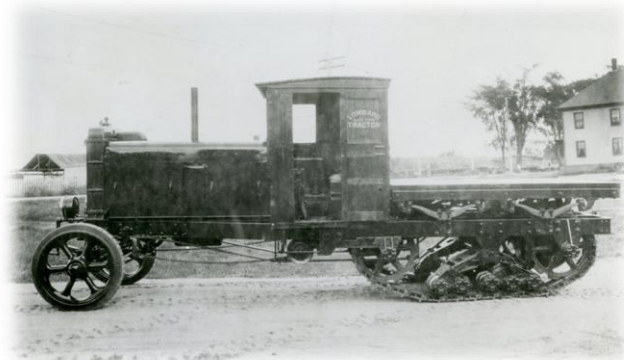
Lombard model GT was rated to carry a 20 ton load. Note heavy leaf springs supporting the platform. Courtesy Donald Johnson
