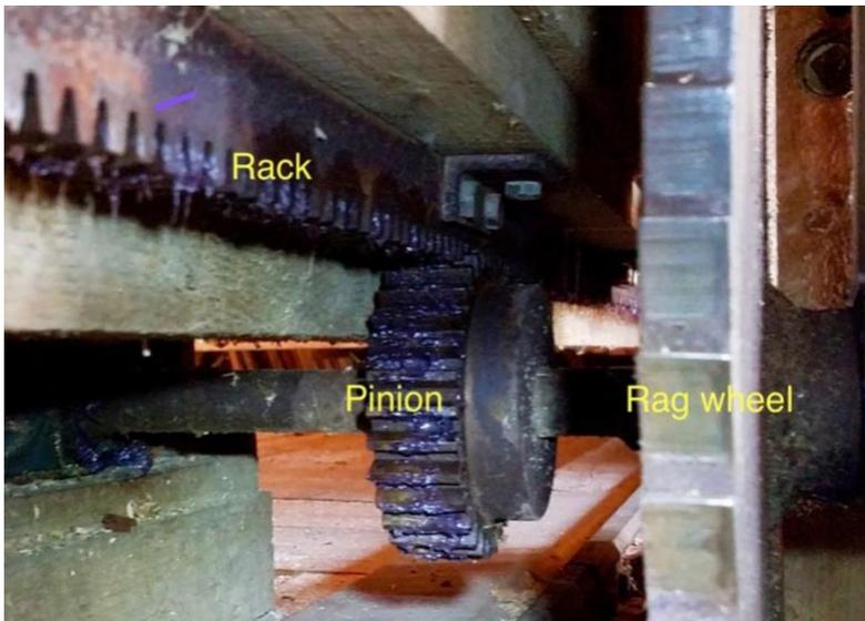
A pusher ratchet turns the rag wheel 6 degrees each time the saw moves up, advancing the log ¼ inch towards the saw blade. A keeper ratchet then locks the rag wheel and carriage while the blade moves down sawing. The pusher ratchet is driven by a wooden linkage connected to the saw frame. You can see the linkage rocking back and forth and hear the steel ratchets clicking during sawing.
