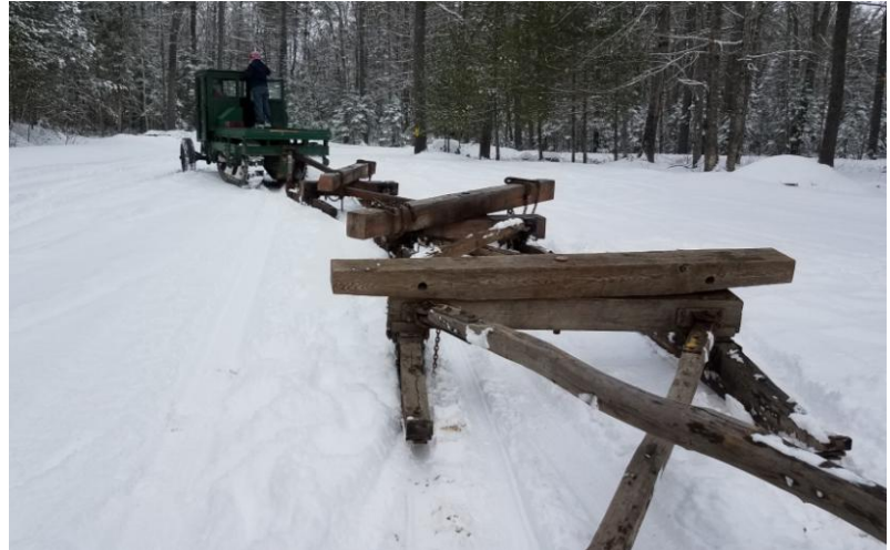
A 10 ton Lombard Tractor-Truck with a set of Lombard patent logging sleds illustrating the method of hooking multiple sleds together using crossed reach-poles. Herb Crosby, Maine Forest & Logging Museum 2022
